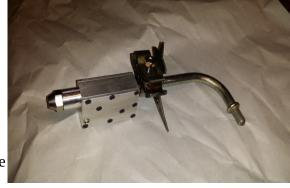
the blast tube. Thread the J-tube into the top port of the preheater block. It doesn't have to be very tight as we are just checking and marking positions.
