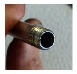
13. Notch the bottom of the electrode holder to make clearance for the cartridge heater wires. You can use an electric grinder, air grinder or even a file. Be sure to to deburr all sharp edges so the wire coverings don't get damaged and short out. You may need to add a chamfer to the other side to give even more clearance for the wires.
