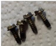
7. Install blast tube with four 1/4" hex head slotted screws. If your burner has an L1 or V1 retention head, you will need to remove the venturi from inside the blast tube. You can either drill out the spot welds
