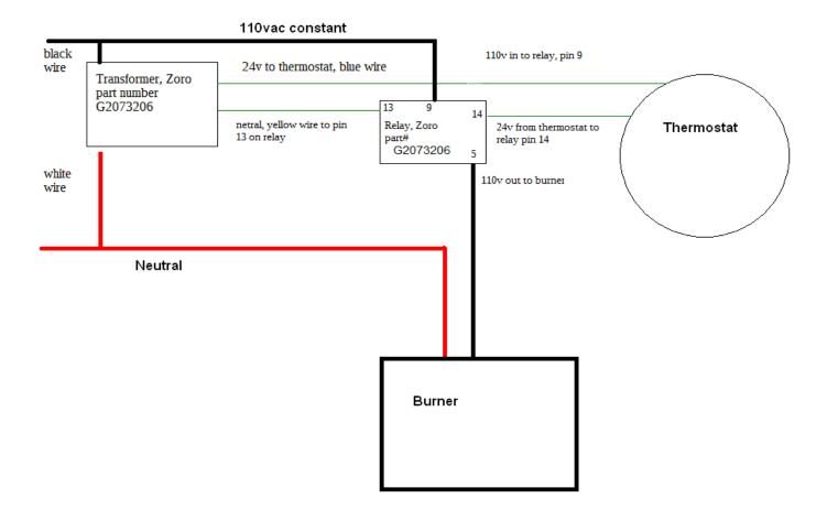
The burner must be wired according to the schematic on page 10. This schematic is only to switch the 110v to the burner using a thermostat and relay. If you are using this on a boiler, the aquastat should already switch the 110v to the burner on a call for heat.
