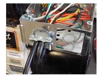
27.Install a wire restraint into the electrical box and insert motor wire and power cord as pictured.
