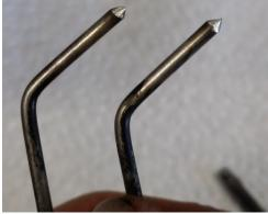
14. Re-point electrodes using a grinder or file. This helps to make the spark more consistent and stable. The points will wear over time.
